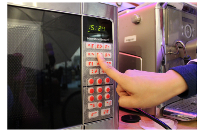
Figure 2: Facade enables blind users to independently create 3D-printed tactile overlays for appliances.
