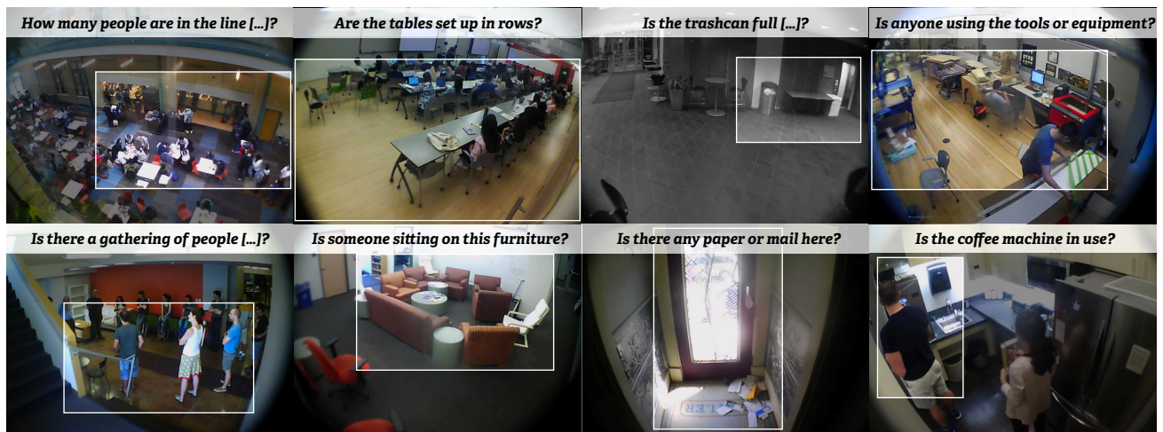
Figure 4: Eight example sensors created by our participants using Zensors++ , with regions of interest highlighted on the full camera image. Many sensors directly complemented and augmented people's existing work practices.
