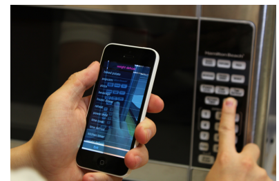
Figure 1: VizLens is a screen reader to help blind people access static physical interfaces.
