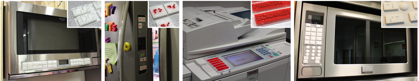
Figure 1. Facade is a crowdsourced fabrication pipeline that enables blind people to make flat physical interfaces accessible by independently producing a 3D-printed overlay of tactile buttons. From left to right, we demonstrate example applications including microwave, refrigerator door, copier, and another microwave. Insets shows close views of individual embossed buttons.
