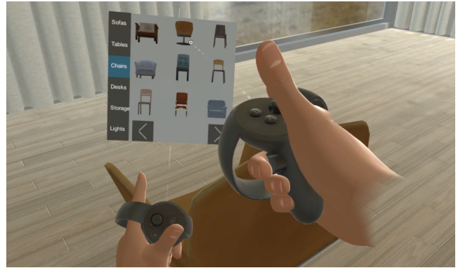
Figure 2: The immersive authoring environment. A menu is always attached to the left controller. Users can select pre-made furniture models of different categories and place them in the VR scene.
