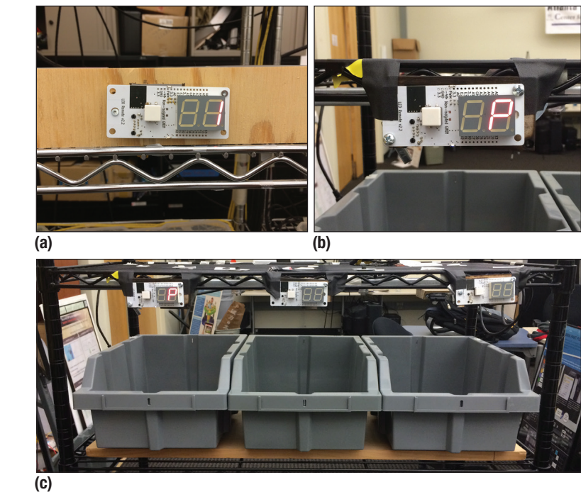
FIGURE 1. Pick-by-light method. (a) The pick bin displays the number of parts to pick (1), while (b) the order bin shows where to place (P) the order. (c) Typically, the order bins are mounted on a wheeled order cart so that the pickers can transport the order bins as they walk through the stacks of pick bins in the warehouse.
