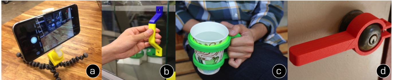
Figure 1: Physically adjustable 3D augmentations accommodate measurement error. From left to right: a tripod mount with ball joint for angle adjustment, an assistive cabinet door handle with a second-iteration update (blue), a cup holder with a flexible ring (light green), and an assistive door lever with an inserted cylinder joint to adjust diameter.
