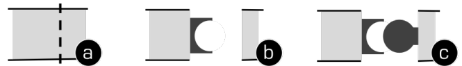
Figure 10: Operations to insert a modular ball joint in a model: (a) Slice the model in two; (b) subtract space to create room for the joint and add the female connector; (c) add the male part.
