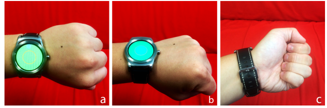
Figure 3. Start and cancel gestures. Using a bubble level metaphor, the user first (a) tilts the wrist, then (b) puts the watch to flat to start the interaction. To cancel an action, the user simply (c) puts the watch to it back.
