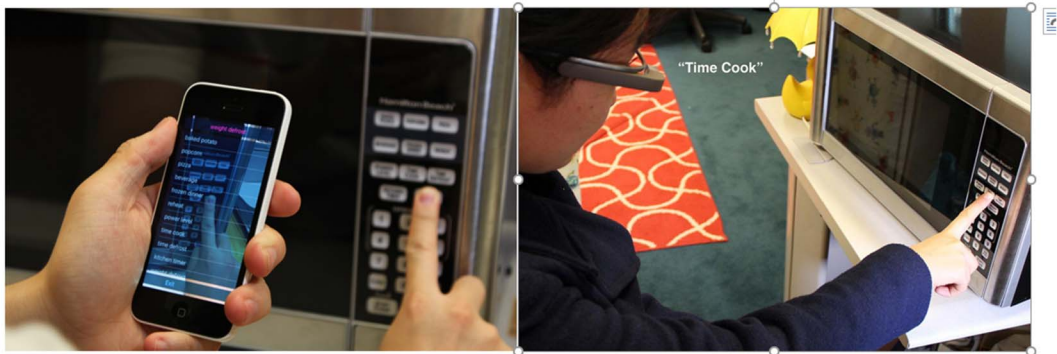
Figure 1. VizLens users take a picture of an interface they would like to use, such as that of a microwave oven. This image is interpreted quickly by crowd workers in parallel. The system then uses computer vision to give instantaneous interactive feedback and guidance on using the interface through a mobile (left) or wearable device (right).
