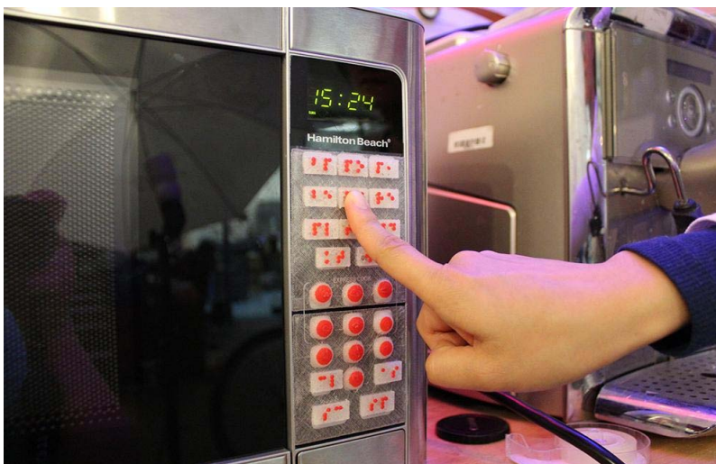
Figure 2. Facade’s crowdsourced fabrication pipeline enables blind people to independently make physical interfaces accessible by producing a 3D-printed overlay of tactile buttons.
