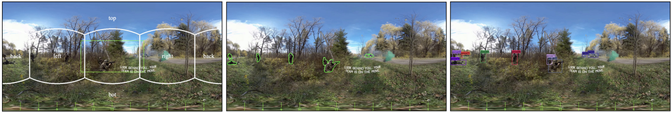
Figure 6: OmniScribe visual overlays: (left) section division outlines the top, bottom, front, back, left, and right. (middle) The visual saliency overlay. (right) The object recognition and tracking overlay.
