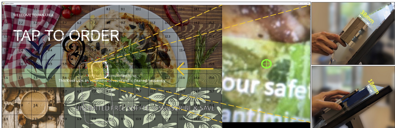
Figure 8: BrushLens maintains a world model of the interface and device location in both the touchscreen interface coordinate (in px) and touchscreen device physical coordinate (in mm). The interface on the left reveals the current state BrushLens calculates, and the image in the middle is the camera view, which has a narrow FoV due to close distance to the touchscreen interface, as shown in images on the right (38mm for the solenoid case and 18mm for the clicker case).
